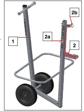
For adaptation to different scaffolding, the machine mounting (2) can be attached by the eye bolt (2a) in three different positions. (Adjustment range 80 mm [31 in] upwards and downwards).
