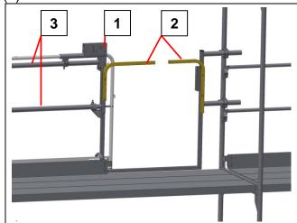
For large scaffold section widths, it may also be necessary to install a horizontal scaffolding pipe (3) to attach the gate.
