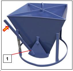
Open flap with lever (1) for unloading.
