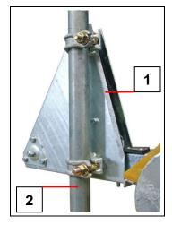
The vertical frame (2) of the scaffolding on which the scaffolding lift is installed, must be aligned vertically.
