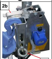
To remove the chassis, open the clamp lock (2b) and pull out the transportation frame (1).
