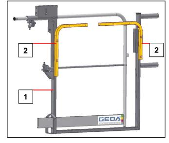
"Simple" loading point protection rails
